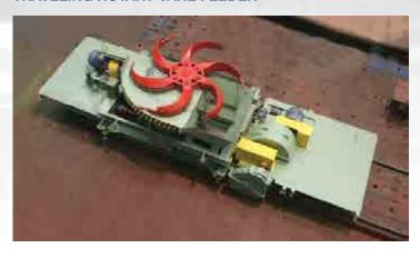
Traveling rotary vane feeder is designed for the uniform feeding of discharge conveyor from the raw-material storage slot hoppers. Transported material: iron-ore concentrate, iron-stone, dolomite, limestone, coal.
