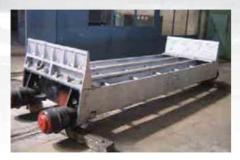
Pallet car is designed for the ore fines and concentrates sintering by the air-sweeping through the charge layer during the sintering belt movement. Car consists of the split body or one-piece steel cast body, four traveling rollers, steel or cast-iron side walls, steel sealing plates and lattice grate. The adoption of seal assembly on rollers allow substantial wear resistance enhancement.
