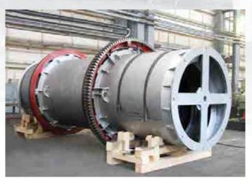
Cooler of sinter returns is a steel welded barrel with internal steel plate lining bearing on four supporting rollers through supporting rings. Two thrust rollers prevents barrel from longitudinal displacement. Barrel rotation is driven by the electric motor through the reduction gear and open gear mechanism, geared rim fastened on one of supporting rings.
