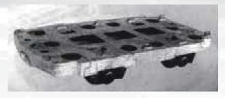
Bogie (TRP 45-4) is designed to transport the molds with scrap from the stockyard to the Martin furnace charging aisle.
