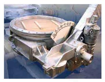
Throttle gas valve is designed to regulate the amount of gas supplied to the gas burner of the furnace stove and complete shutoff of the burner from the gas main during normal operation or when the current fails. The valve is installed on vertical section of the gas main.
