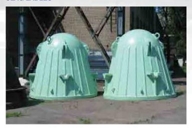
Slag ladle is designed for collection of molten slag discharged from furnaces, steelmaking and ferroalloy units. The ladles are filled with the slag with temperature of up to 1600°C and density of up to 3,7 t/m<sup>3</sup>.
