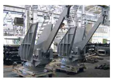
Bleeder stacks of DN250 and DN400 types are designed to discharge gas from the dust collector into the atmosphere. The bleeder stacks are installed on vertical sections of the gas bleeders. Bleeder stack of DN800 type is designed to discharge gas from the dust collector into the atmosphere. The furnaces are usually equipped with two such bleeder valves installed in the upper parts of the gas bleeders.
