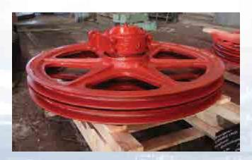
Rope sheaves are designed to direct the ropes of the blast-furnace skip hoist.
