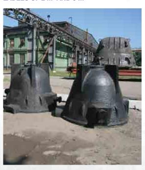
The ladles are designed for collection and transportation of molten slag with temperature of up to 1500°C.
