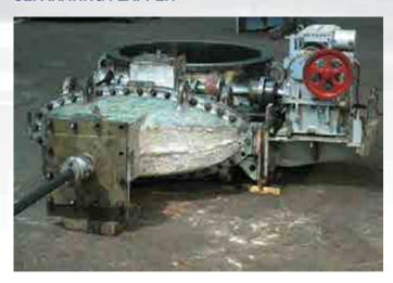
Separating flapper is designed to quickly shut off the flow cross-section of the mixing cold blast pipe in case the blast supply to the furnace is stopped in order to prevent the possibility of penetration of hot gases from the furnace to the cold blast pipe. The flapper may operate in the automatic control system.
