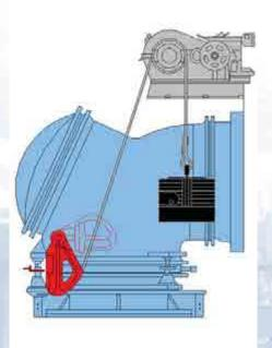
The fume valve consists of: housing, cover, plate and cooled seat.
