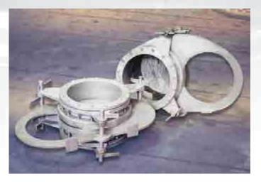
Goggle valves of DN350, DN500 types are designed to completely shutoff the equalizing valves of the charging gear from the working chamber when the maintenance operations or revisions are held. The valves are installed on vertical sections of the mains. Goggle valves of DN1100, DN1300 types are designed to completely shutoff the stoves from the gas mains and air mains coming from the central ventilation station of the air mains when the maintenance operations or revisions of the stoves are held.
