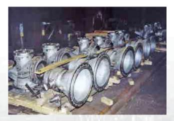
The tuyere connections are installed directly near the furnace connecting it to the hot-blast circulating duct.
