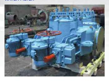
Water filter is designed to perform primary mechanical purification of water, fractions over 6,3 mm, supplied to the blast-furnace cooling system. The filters may be supplied either with a hand or electric drive.
