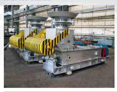
Screw dust unloader is designed to humidify and remove the dust from the dust collector of blast-furnaces and simultaneously suppress the fine dust.
