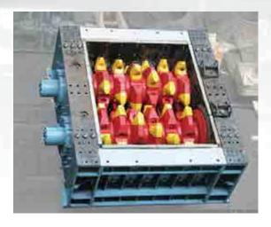
Toothed screw crusher is designed for loading of mined rock with the maximum feed size up to 1500 mm (Protodyakonov hardness up to 15) and its crushing to the output size of 300 mm. A crusher is installed at the coarse crushing stage.
