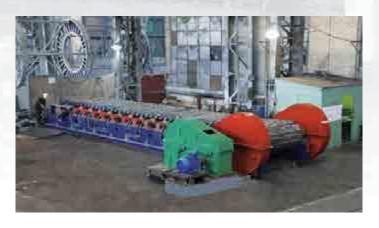
The main advantages and structural features of the feeder plate: simplicity and reliability; possibility of continuous operation mode; the ability to install angle of 15°.
