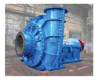
Pumps NP-800-2M and NP-500M are centrifugal barrel insert pumps with the vertical discharge manifold. Pumps are intended for pumping of abrasive water mixtures. Pumps are used at ore mining-and-processing integrated works.
