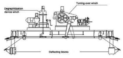
The turning- over mechanism is intended for control of heating gas reversing cocks of reversing valves and the valves of the decarburization during change of gas and air flow direction to the heating system of the coke (coked pitch) ovens and disposal of burning products. The mechanism consists of the rods connected with turning-over winch (turning-over device) and the winch of the degraphitization device.
