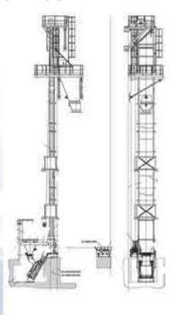
Intended for hoisting the under –leveler charge formed when leveling by the coke pusher. The under-leveler charge is delivered from the hopper installed on the coke pusher to lower hopper of skip hoist. The charge is transferred from the lower hopper of skip hoist to the upper one. From the upper hopper the charge is periodically unloaded to the last hopper of coal charging machine.
