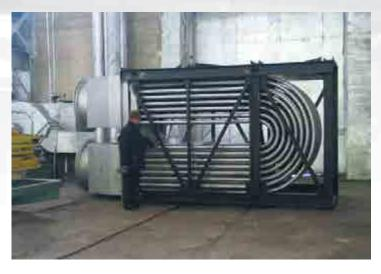
Tubular loop recuperators are designed to recuperate heat of the waste combustion gases with temperature of up to 1000°C and to heat the air available in furnace units for fuel combustion up to 350-400°C.
