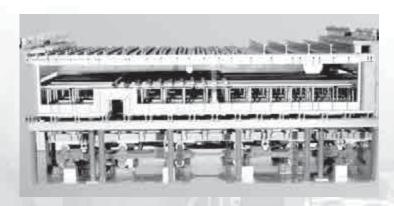
Reheating furnace with walking beams is designed for heating or heat treatment of stocks made of carbon, alloyed and special steel before rolling. Metal is heated in the furnace with different heating devices during the radiating low-oxidation and low-decarburization heating process.
