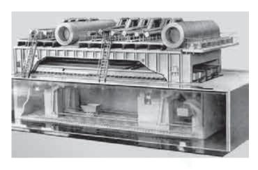
Reheating furnace with walking hearth is designed for heating or heat treatment of stocks made of carbon and special steel and of alloys before rolling. Metal is heated in the furnace with flat-flame burners during the radiating low-oxidation and low-decarburization heating process.
