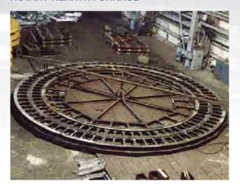
Rotary hearth furnace is used in pipe rolling and is designed to heat the ingots before rolling. The furnace hearth travels along the supporting rolls. The centering rolls are applied from the lateral hearth travel. The hearth consists of the upper and lower rings made of segments. The furnace is equipped with water-sealed valves arranged at the inner and outer hearth diameters.
